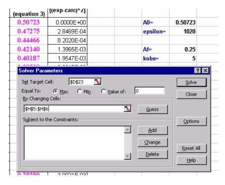
On **Solver Parameters** click on **Options.** Change **Max Time** to **1200 seconds** (kinetics run time). Click **OK**.
