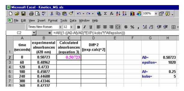
To fill cells C3 through C22, click on cell C2. Bring the cursor to the right low corner and press left mouse and drag all the way down to cell C22. Depress the left mouse. All cells (C2:C22) should now be filled in with the calculated ("crude") Absorbances:
