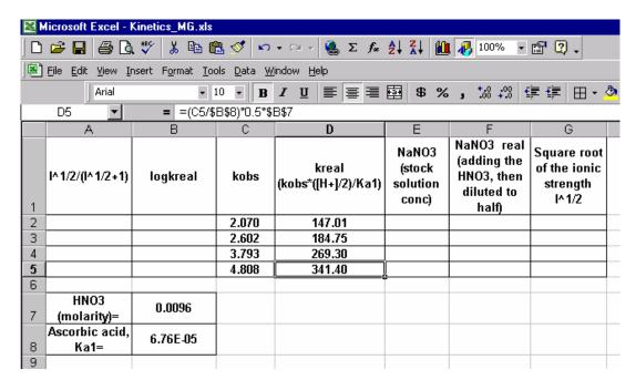
5. Calculate logkreal in cell B2 as LOG10(D2). Drag the cell content as described above down to B5:
