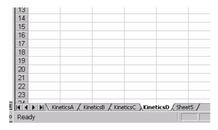
4. Add your experimental data to the four sheets. For example **Kinetics\_B** sheet is shown below. Type in column A, the **time** (in seconds), and in column B the **experimental absorbances** (@420nm) corresponding to the respective time. Add two more columns. One for **calculated absorbances** (from equation 3) and one for the **square** of the difference, i.e., **experimental absorbances** (**column B**)-calculated absorbances (**column C**).
