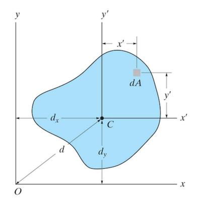
**Note:** the integral over y' gives zero *when done through the centroid axis*.
