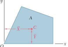
In the case of a composite area, we divide the area A into parts  $A_1$ ,  $A_2$ ,  $A_3$
