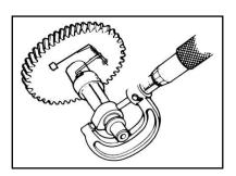
**NOTE:** If this measurement is out of specification, complete engine replacement is required. The only internal parts available for this engine are gaskets and seals.
