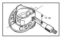
**NOTE:** If this measurement is out of specification, complete engine replacement is required. The only internal parts available for this engine are gaskets and seals.
