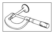
**NOTE:** If this measurement is out of specification, complete engine replacement is required. The only internal parts available for this engine are gaskets and seals.
