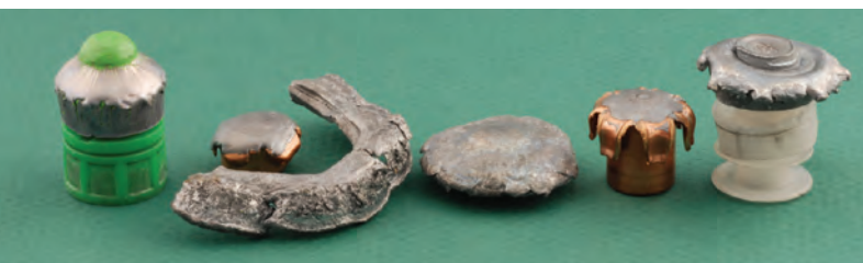
Above at left, the Brenneke® Green Lightning compared to several competitive rounds after firing into ballistic gelatin. Note the excessive expansion of the other slugs compared to Brenneke. This can mean insufficient penetration and a wounded animal.
