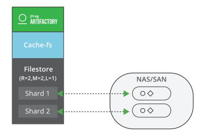
The redundancy must be less than or equal to the number of mounts in your system for Artifactory. If the number of writes specified by the redundancy is not reached (mount failure for example), the WRITE transaction will fail.
