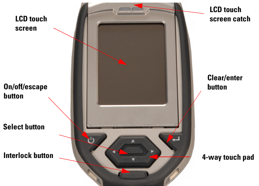
Figure 0-2. The Control Panel
