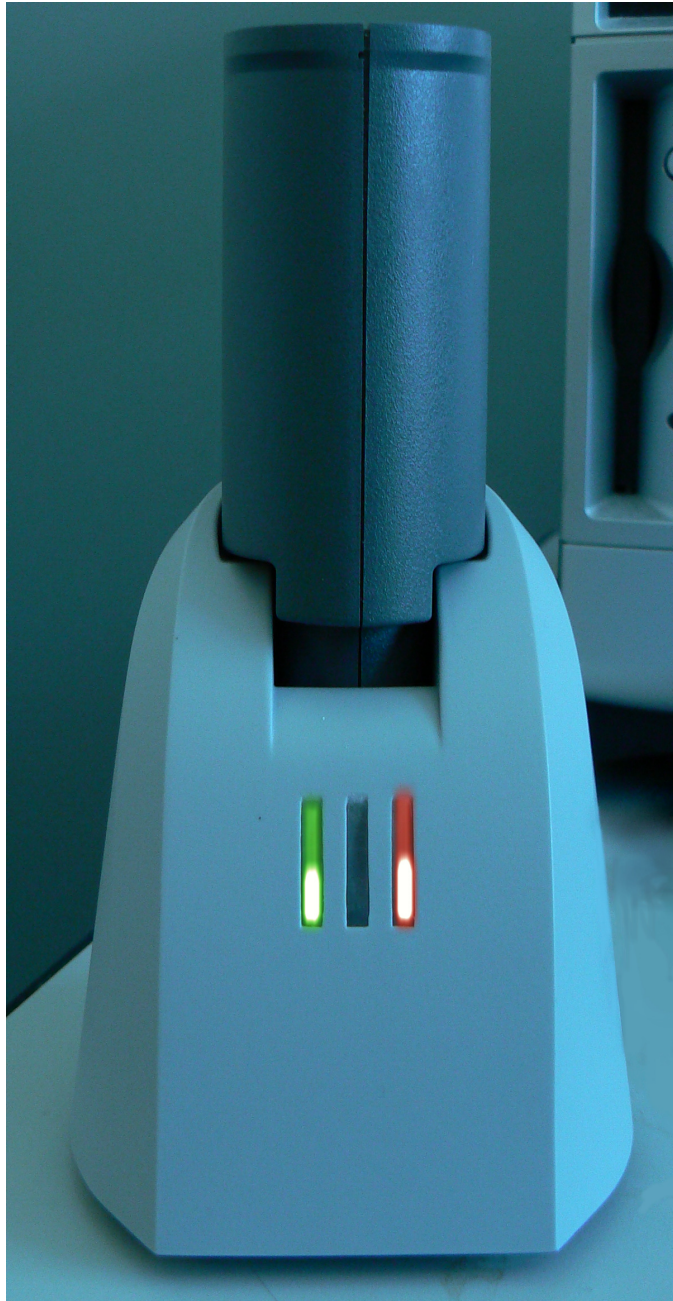
Figure 2-4. Battery Pack in the Charger
