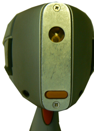
Figure 2-5. View of Face Plate and measurement window
