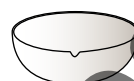
evaporating dish: used to evaporate off the solvent from a solution, leaving crystals behind
