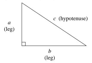
Note that the hypotenuse *must* be c. The hypotenuse is the longest side, and is always opposite the right (90°) angle. It makes no difference which leg is a and which leg is b.
