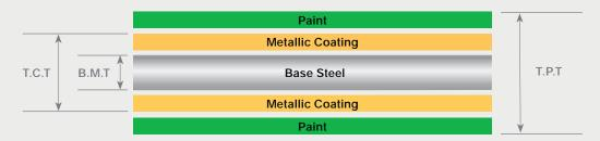
When ordering through different suppliers or importing sheet & coil products, it is important to understand the difference between B.M.T., T.C.T. & T.P.T.
