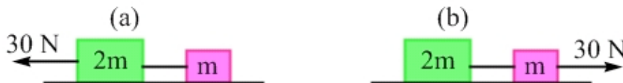
Figure 3.26: Two situations involving two boxes on a horizontal surface. The boxes are connected by a string of negligible mass. For Exercises 29 and 30.
