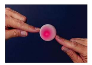
a) Place a finger of each hand on each of the two metallic electrodes on the Energy Ball. Describe what happens.
