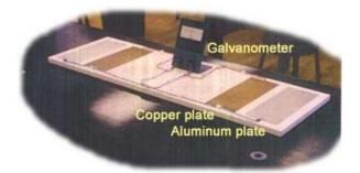
a) Examine the "Hand Battery." Describe the construction of this device as best you can. Use a sketch if necessary.
