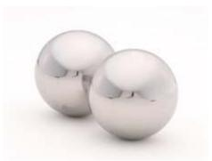
a) Place a piece of paper between the two spheres. Now smash them together. After the spheres collide, smell the area on the paper where they came into contact. What do you detect? What do you suppose caused this odor?
