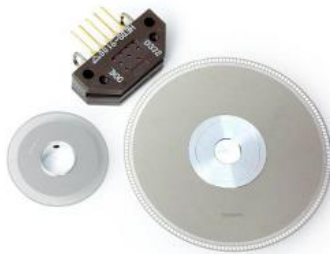
Fig. 1: The Avago Technologies HEDS-9040/9140 series of three-channel optical encoders can work with resolutions up to 2000 ppr, and the vendor offers a family of suitable code wheels as well, with different diameters to enhance the resolution readout.
