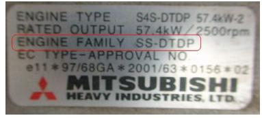
If the engine label does not list the U.S. EPA-issued engine family name, the manufacturer of your engine may be able to assist you in determining the engine family name if you are able to supply information on the model year and make of the engine, or the engine serial number. Some manufacturers also have online tools where their customer can enter engine serial numbers and determine the engine family name.
