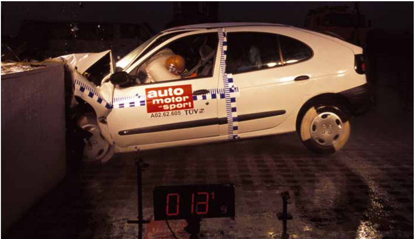
Figure 11.5 In this test the dummy is protected by an airbag, and the crumple zone at the front of the car allows time for the passengers to slow down.
