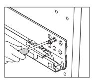
Once your outer drawer slides are in, fit your inner drawer slides. The inner drawers slides are fitted to the inner row of holes in your cabinet.
