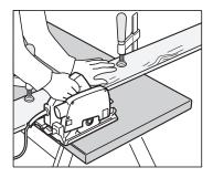
Use a circular saw and G clamps to hold a straight-edge to your pre-cut benchtop when you cut to customise the size. It's useful to use a pair of sawhorses to help you. A tip is to have a second person holding the piece to be cut off to prevent the edge from splintering.
