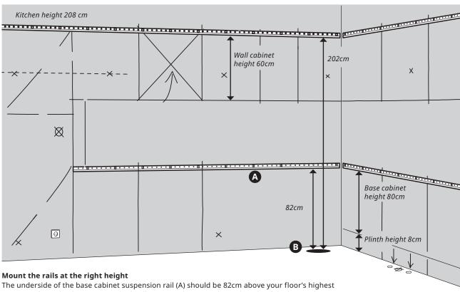
The underside of the base cabinet suspension rail (A) should be 82cm above your floor's highest point (B). If your kitchen is 208cm high, allow 120cm between the underside of the base cabinet suspension rail and the underside of the rail for the wall/high cabinet. If the kitchen is 228cm or 248cm high you should allow 140cm or 160cm respectively.
