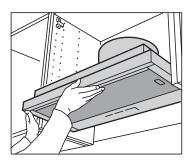
Install the rangehood. IKEA rangehoods can be installed in two ways: either ducted to the outside, called extraction; or used in recirculation mode fitted with a charcoal filter. Each installation option is described in the assembly instructions that come with the product.
