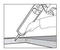
To prevent moisture from penetrating the benchtop apply polyurethane silicone across the sawn edges.
