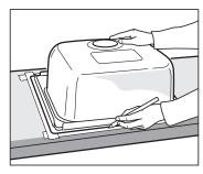
Mark a spot for the sink by laying the benchtop in place. Trace the inside of the base cabinet onto the underside of the benchtop. This helps you align your sink. Turn your benchtop over and trace the outline of your sink onto masking tape.
