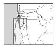
Place the newly cut edge of the filler piece against the wall —it should fit perfectly. Mark the edge of the cabinet on the top and bottom of the filler piece. Draw a straight line from these points and cut.
