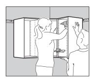
Hang the corner cabinet first and secure by tightening the screws. Hang the remaining cabinets and connect them with the included screws. Wait to tighten the screws until the base cabinets are in place and you can ensure alignment.
