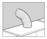
Saw the hole either in the back panel or in the top of the cabinet, following the assembly instructions. For safety and functionality, use the exact measurements that are recommended in the instructions for installation of the rangehood.
