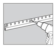
Fasten your rails, base cabinet rails first. Make sure you've found suitable points in the wall where the rails can be fastened, and that the rails are level before drilling.
