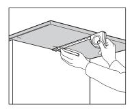
Proof measure your benchtop. If you have a pre-cut benchtop now is the time to cut it to the right length. Cut with the benchtop underside facing up if you are using a buzz or jigsaw, but with the top facing up if using a handsaw.
