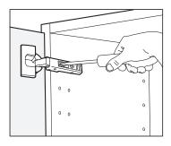
Align your doors to the correct height and width by adjusting the screws on the hinge plate.
