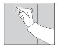
Check your wall is strong enough to hang your suspension rail and cabinets. Depending on your wall material, it's best to install your rail onto a stud or a support beam. Using an electronic stud finder can be helpful.
