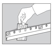
If your wall is uneven use distancers between the rail and the wall to make sure the rail is straight.
