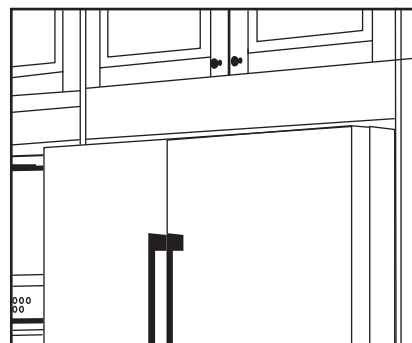
Fillers: to be cut from ½" or ⅝" thick cover panels to create the filler needed in your design. For filler above the fridge, use a 5" high drawer front
