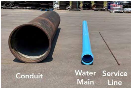
There are typically three pipe sizes used to deliver water to customers. Conduits carry large amounts of water over long distances. Water mains branch off the conduits and run into neighborhoods. Service lines are owned by customers and connect homes and businesses to the water mains.
