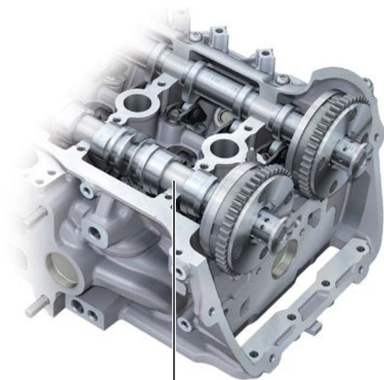
EA888 Generation 3 Camshaft bearing journal on the AVS cam element
