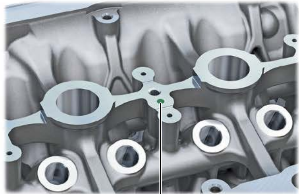
Oil drain channel from fine oil separator
