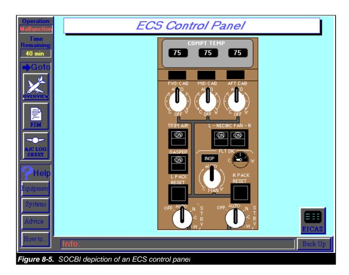
Students use the working controls and displays to practice diagnosing a number of (usually randomly occurring) faults built into the simulation. **SOCBI** modules also contain diagrammatic, i.e., logical, representations of the system being taught. An example of these diagrams is shown in **Figure 8-6**. These functional/logical diagrams teach students how a system is functionally connected and allow them to use logical troubleshooting algorithms such as half-splits.
