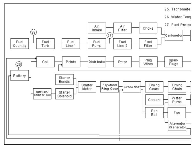
Figure 8-3. A logical troubleshooting diagram for an automobile engine
