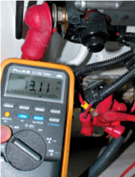
Left: This DMM is being used to verify that battery voltage is available at the starter solenoid's primary terminal. This starter solenoid is an auxiliary and is remotely mounted, many are attached directly to the starter. Right: This alternator is not charging and the DMM tells the whole story. Connected to the alternator's output stud, the voltage is a mere 12.3 volts, well under a properly operating alternator's expected output of 13 or more volts.
