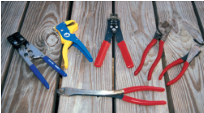
Left: The right tool for the job, a good set of wire cutters, crimpers, and strippers are critical for proper electrical repairs. Right: One of several automatic wire strippers that are available, these are nearly fool-proof and ideal for those who strip wires infrequently.
