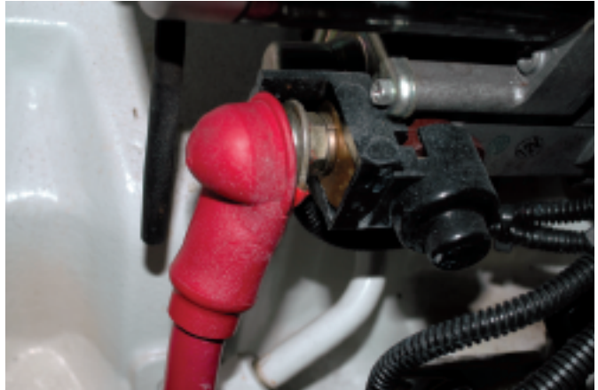
Left: An auxiliary starter solenoid is mounted remotely from the starter itself, so you may have to follow the large, secondary wire from the starter to locate it. It's usually not more than a foot or two away from the starter. Right: The secondary output from a starter solenoid is always a large cable, usually the size of your pinky or larger. When it's energized, the starter should be turning.
