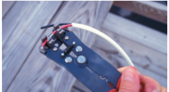
Left: The right tool for the job, a good set of wire cutters, crimpers, and strippers are critical for proper electrical repairs. Right: One of several automatic wire strippers that are available, these are nearly fool-proof and ideal for those who strip wires infrequently.
