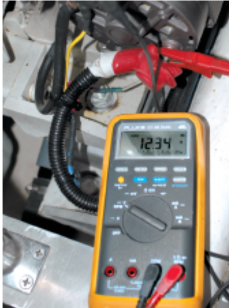
Left: This DMM is being used to verify that battery voltage is available at the starter solenoid's primary terminal. This starter solenoid is an auxiliary and is remotely mounted, many are attached directly to the starter. Right: This alternator is not charging and the DMM tells the whole story. Connected to the alternator's output stud, the voltage is a mere 12.3 volts, well under a properly operating alternator's expected output of 13 or more volts.
