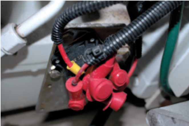
Left: An auxiliary starter solenoid is mounted remotely from the starter itself, so you may have to follow the large, secondary wire from the starter to locate it. It's usually not more than a foot or two away from the starter. Right: The secondary output from a starter solenoid is always a large cable, usually the size of your pinky or larger. When it's energized, the starter should be turning.
