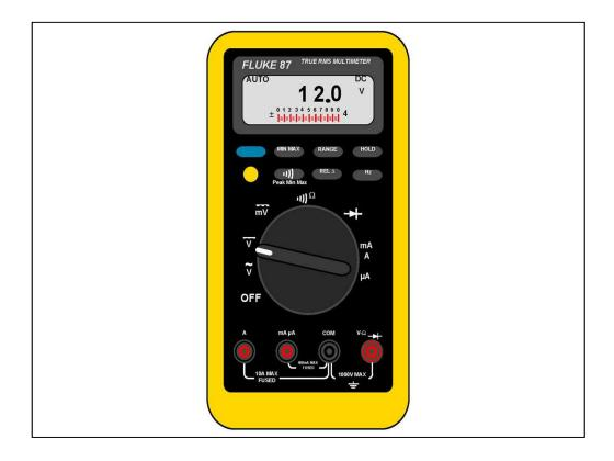
When using the multimeter to make voltage measurements it is important to remember that the voltmeter must always be connected in parallel with the load or circuit under test. The accuracy of the multimeter is approximately  $\pm$  0.01% in the five ac/dc voltage ranges with an input impedance of approximately 10 M $\wedge$  when connected in parallel.
