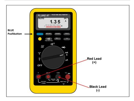
When using the multimeter to make current measurements it is necessary that the meter probes must be connected in SERIES with the load or circuit under test. To toggle between alternating and direct current measurements, use the BLUE pushbutton.
