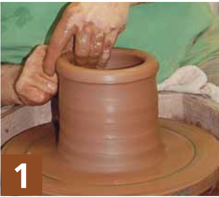
1 Throw two identical jars. It is easier to match jars when you make a lot.
