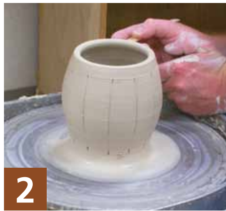
2 Mark an evenly spaced grid around the exterior.
