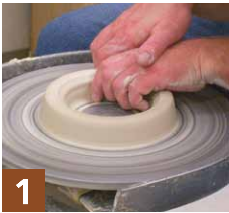
1 Throw a basic cylinder without a bottom.
