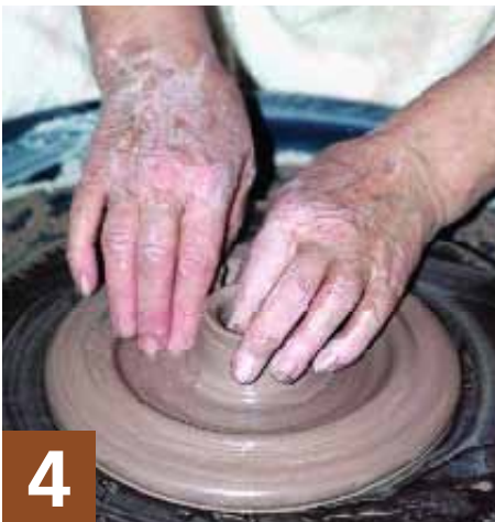
4 Pull up wall of center opening.
