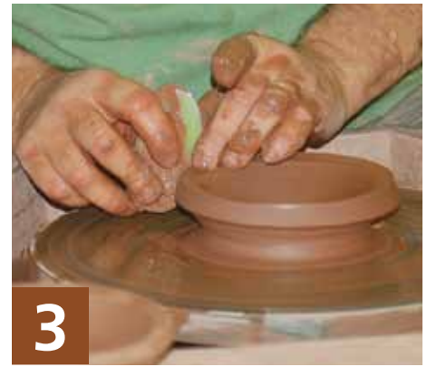
3 Make lids with a slight inward bevel on the rim.
