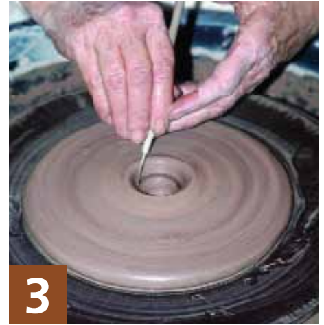
3 Trim inside opening with a needle tool.
