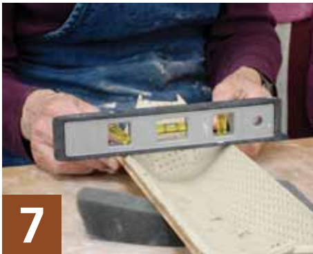
7 Prop the piece up, level the sides, and adjust as needed.
