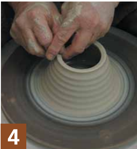
4 The top should be slightly wider than the opening of the body.
