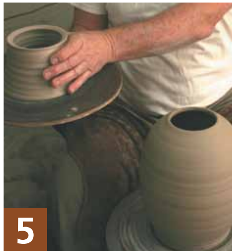
5 Carefully move the top to the body.
