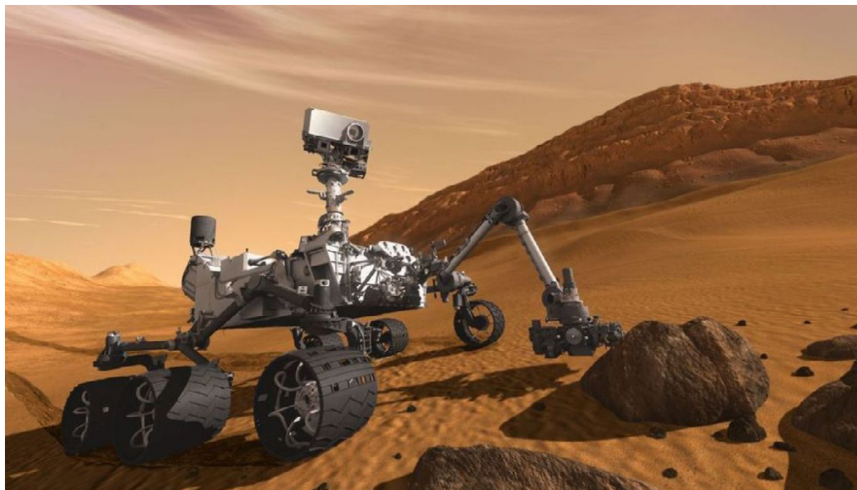
The Mars Rover is powered by plutonium, another legacy of the Manhattan Project
