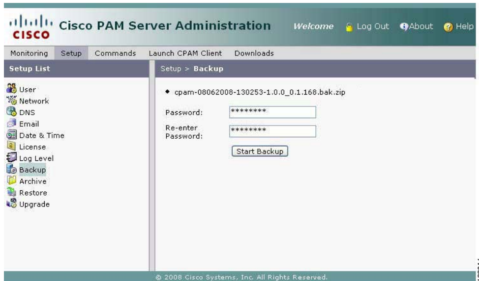
Figure A-1 Backup Window in the Cisco PAM Server Administration Utility
