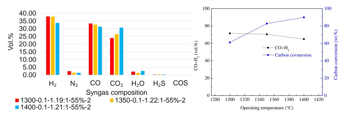
• The H<sub>2</sub> content decreased with the increasing operating temperature but are higher than the contents of CO and CO<sub>2</sub> for all three conditions.
