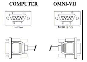
The serial port of the OMNI-VII is defined as a DCE terminal. Which means that it is meant to be connected to a Computers DTE terminal. Using a straight through RS-232 control line. If you wish to control another serial device, and if it is a DCE terminal type of a device also, then the cable you need to use is a null-modem RS232 Interface cable. If
