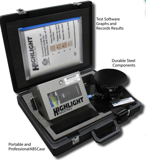
The Portable Film Force System is the best way to measure and record film performance in the field.
