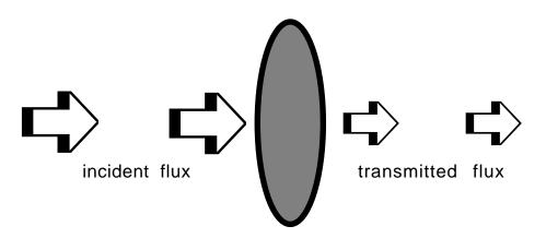
The <u>transmittance</u> or <u>transmission</u> of a lens is the ratio of the light that goes through it to the light incident on it,
