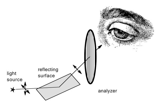
The diagram shows how an unpolized beam of light is polarized by a reflecting surface such as a road bed or body of water and the now horizontally polarized light is prevented from reaching the eye by the vertically polarized sunglass lenses.
