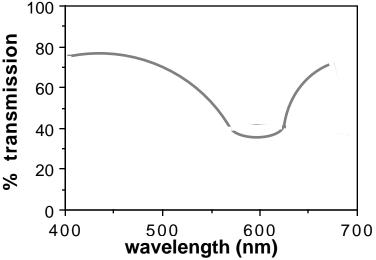
The transmission curves of blue filters show great attenuation of the long wavelengths of visible spectrum.
