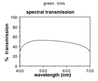
The figure shows the transmission curve of an idealized green tint. Note the peak of the curve shifted towards short wavelengths.
