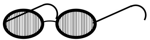
The figure above indicates that polaroid sunglasses contain vertical polarizing filters.
