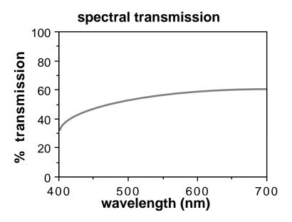
The figure shows the spectral transmission of a typical brown lens. Note the almost linear rise from ultraviolet to infrared.
