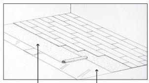
Foam to be used only with flooring Vapor barrier over concrete planks that do not have attached underlayment.
