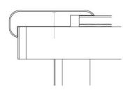
edge with a nosing. The illustration at right shows square edge nosing with Pergo on the edge, and installed Pergo on the tread and riser with a nosing finishing the nose of the tread.
