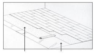
Foam to be used with only with flooring planks that do not have attached underlayment.
