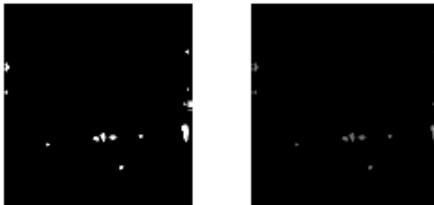
Fig. 7. Plot image segmentation result in the visible domain: Calcite against not calcite segmented image (left) and infiltration severity degree map (right)
