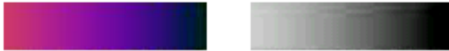
Fig. 8. The cold temperature part of the infrared scale: Original (left); its red component (right)
