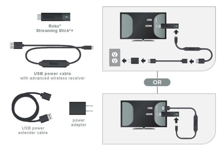
To get started, connect your Roku Streaming Stick+ to an available HDMI port on your TV. If you plan to stream movies and TV shows in 4K or 4K HDR, remember to select an HDMI 2.0 port that supports HDCP 2.2. Learn what to look for when trying to identify an HDMI input that supports HDCP 2.2.
