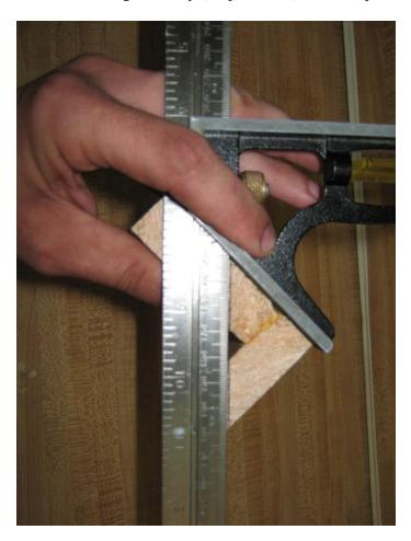
Place it on the end of the part as shown, and trace a line, leaving a space of about 1/4" (it's not critical) between the square and the internal apex of the angle.
