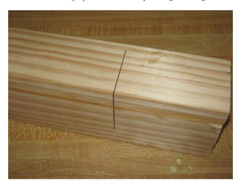
Now, make a mark on each of these lines, at the distance you measured earlier (1 7/8" in my case) from the apex's edge. Make another mark on the apex's edge, 5 1/2" from the lines, and trace a diagonal between the marks.
