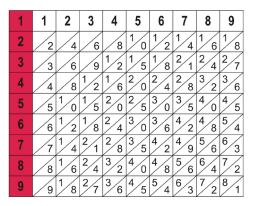
Napier bones-Numbers 0 to 9 were marked on a set of ivory sticks in such a way that the product of any number can be found by placing the sticks side by side.
