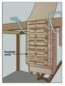
Jyoti: The Jacquard loom invented by Joseph Marie Jacquard used punched cards to control a sequence of operations. A pattern of the loom's weave could be changed by changing the punched card.
