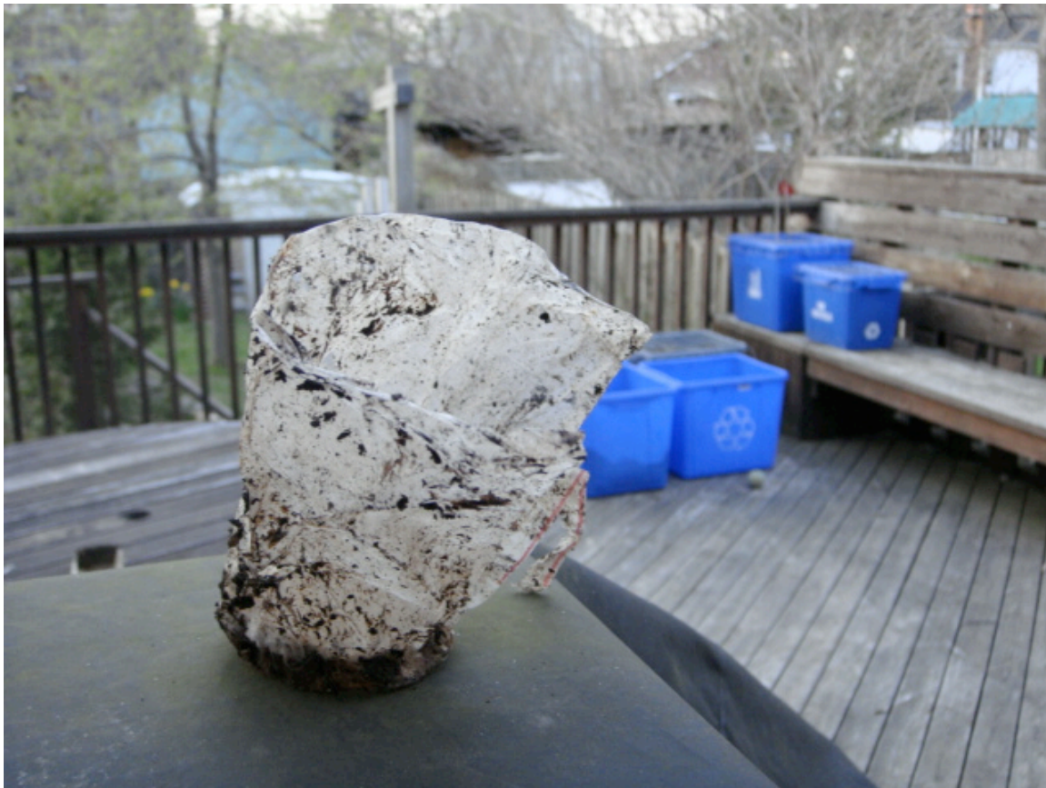
Figure 1: An industry standard 'poly lined' paper cup retrieved from over a year in a residential compost.
