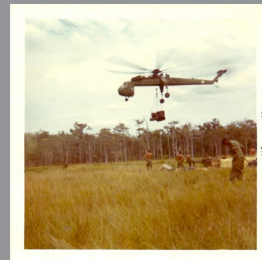
35. Larry Diesburg, Ch-54 Tarhe Skycrane Dropping Dozer At Lz, Near Tay Ninh, Vietnam
