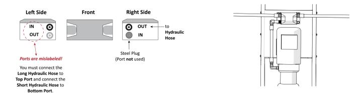
If your Flow Divider looks like the graphic below, **rotate the Flow Divider 180°** so that the side with an **IN** and **OUT** Port is on the *right* side, and then connect the Short Hydraulic Hose to the Lower **IN** Port; the other end of the Short Hose connects to the Pressure Port on the right side of the Power Unit..
