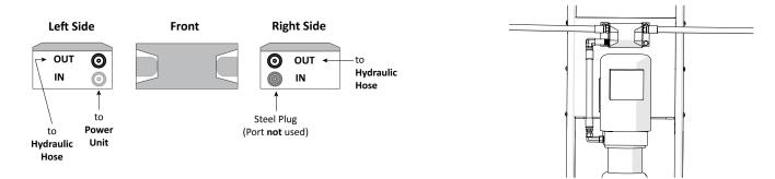
If your Flow Divider looks like the graphic below, the Left side Ports are **mislabeled**. *Do not connect the Short Hydraulic Hoses to the Top Left Port*. Connect the Short Hydraulic Hose connects to the Bottom Left Port, and two Long Hydraulic Hoses connect to the Top Ports on either side of the Flow Divider.
