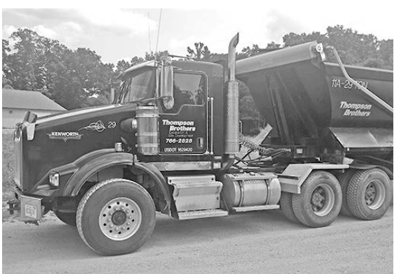
'06 KWT800, 565 hp Cum., 423,000 miles, 18 spd., 20F, 46R, wet kit, dbl. plumbed, $65,000 or best offer. (231) 206-5307
