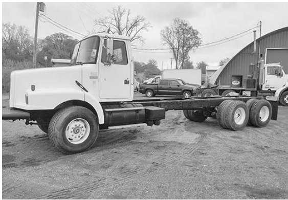
'99 Volvo WG64 tdm. axle C&C, N14 Cum., 9 spd., 18F, 40R, dbl. frame, Hend. susp., $19,500. (616) 836-5691
