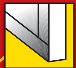
Triple folds on the long edge of doors for safety and strength.
