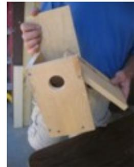
back into the top piece. Now all we need to do is drill the hole through either the front or back to lock the opening side in place with a 6d duplex nail and drill a 1/2" hole, 1 1/4" down from the top of the back in the center to mount the house.
