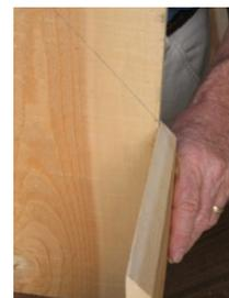
3. Cut one piece 8" x 7 3/8" for the floor. Remember, you always want to enclose the floor with the front, back and sides.
