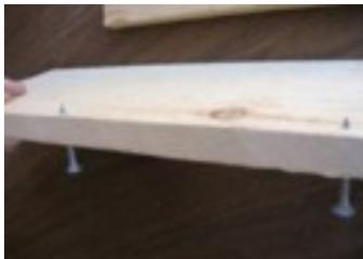
so that just the tip of the screw comes through the board. Then line up the tips of the screws with the pre-drilled holes in the side piece and drive
