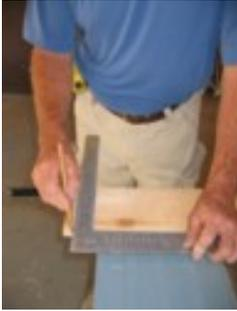
any bad wood from the end of the board. Use your T-square to mark a straight line across your board. You can use a table saw if you have one, a circular saw or a hand saw. Make sure if you are using any type of power saw that you follow the manufacturer's instructions
