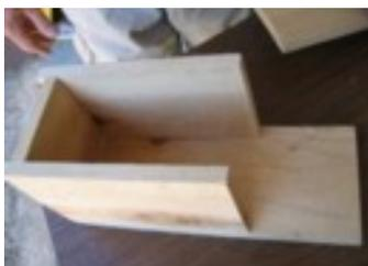
screws about an inch from the top and bottom. If you are using the slot entrance make sure you place the slot at the top of the house. Notice in the picture above that the floor
