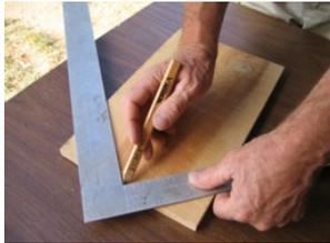
center of the front piece so each slope measuring 5" from the peak to the edge. Then find the middle of the front on the bottom and measure 1 1/2" toward each edge and make a mark. This will give you a 3" wide bottom and when you measure from where your roof meets the edge, to your mark on the bottom, you should have about 6 3/8" sides. Make the same measurements and cuts for the back piece.
