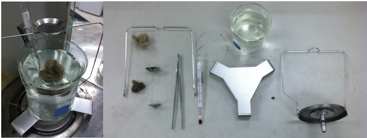
Figure 3. Mettler Toledo 33360 density determination kit.
