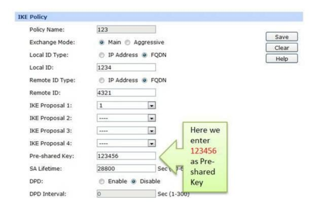
NOTE: No matter on Main mode or Aggressive mode, once the client PC is behind a NAT device, we have to select FQDN as ID Type and the NAT device must support VPN passthrough, otherwise the VPN tunnel can't be established.
