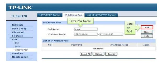
NOTE: IP Address pool must be different range from LAN IP address range.
