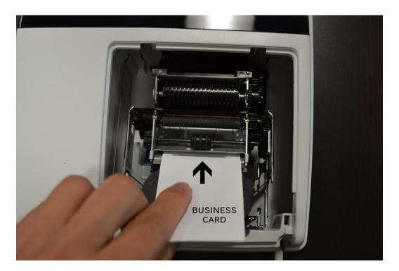
2.2. If you're able to push the paper through using the business card, use a needle nose plyer to pull the paper from the other side, as seen in the below image.
