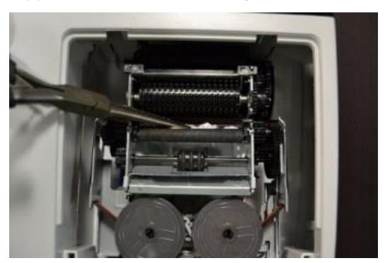
3. Note: this step is only necessary if there is plenty of paper sticking out from the printer feed. As seen from the image below, use plyers to carefully pull the paper out from the printer feed.
