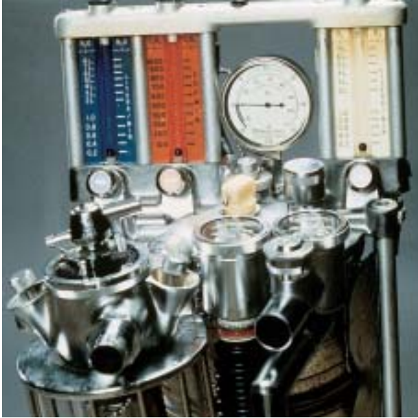
Fig. 31-18. Military Field Anesthesia Machine Model 785. The ether/chloroform in-circuit vaporizer is seen at bottom left. Flowmeters, seen left to right, are for nitrous oxide (blue), cyclopropane (orange), and oxygen (white, the international color for oxygen). A pressure gauge, calibrated in centimeters of water, monitors the pressure in the breathing circuit. Immediately below the pressure gauge is a round button, the oxygen flush valve. Two one-way valves for the breathing circuit can be seen at the bottom right. The white plug with a small chain attached, seen in the center of the photograph, can be removed and replaced by the hand-operated concertina bellows (also see Figs. 31-19 and 31-21). Photograph: Courtesy of William Clayton Petty, MD, Captain, Medical Corps, US Navy, Bethesda, Md.
