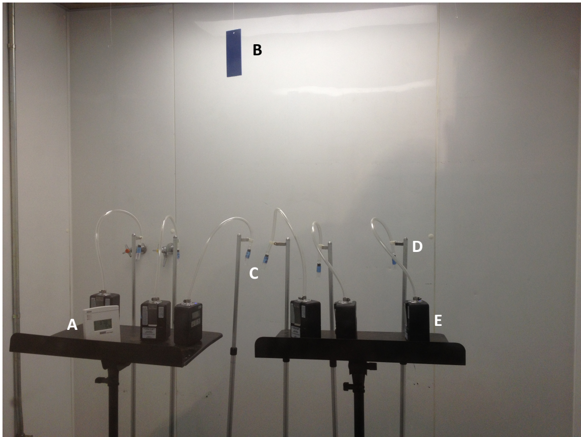
Figure 3: Equipment setup with in the experimental space. Pictured is the (1)-65 g Nuvan Prostrip+ experiment. (A– HOBOTermometer/Humidity Meter, B – Nuvan Prostrip+, C – Sampling Media, D – Sampling Stand, E – Personal Air Sampling Pump)
