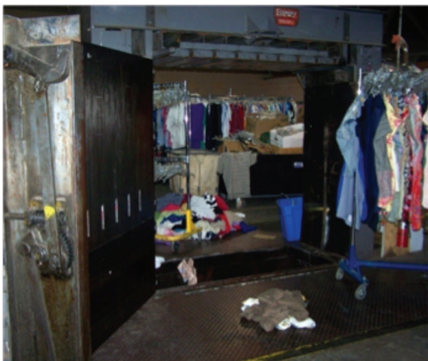
Figure 1. A steel baler with a deep pit compacts unwanted textiles into bales.
