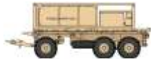
M1076 TRAILER PLS 8X20 W/LOAD HANDLING SYSTEM 2000GAL CAP WATER TANK (HIPPO)
