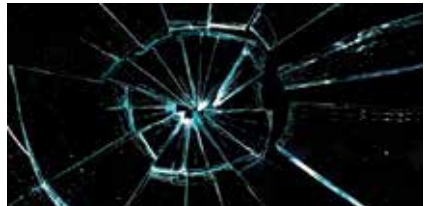
Cracked glass greater than 1/2" in diameter or spidered cracks
