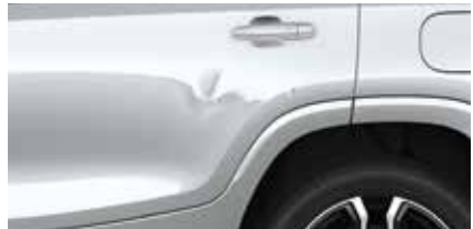
Hail damage or punctures on any panel
