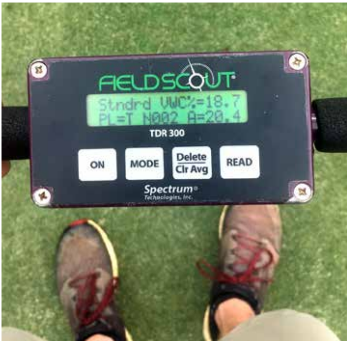
Soil moisture sensors and other irrigation management tools inform good irrigation decisions. Photo credit: Tim Busek.
