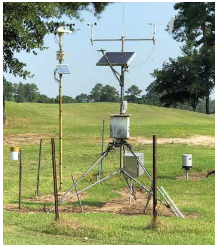
On-site weather stations access weather information and ET rates to determine site-specific water needs. Photo credit: Lukus Harvey.
