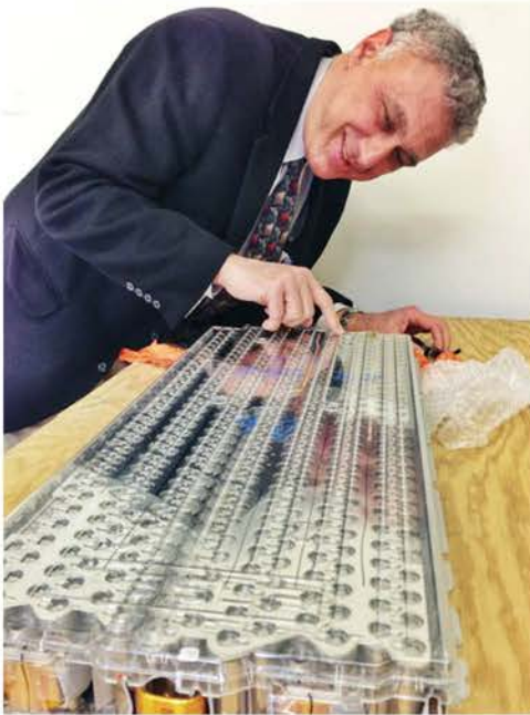
Tesla Module (85 kWh Model S) with 444 individual cells
