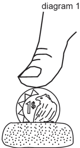
coin pressed on the edge sinks into the plasticine
