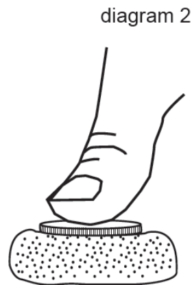
coin pressed on the flat surface does not sink into the plasticine
